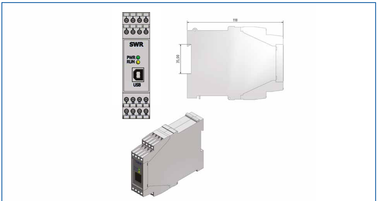
Fig. 2: DIN Rail transmitter dimensions
