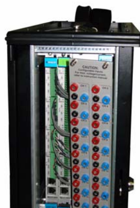
(d) Rear view showing installation of panel for banana connectors
