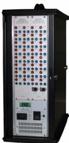
(e) Banana connector panels installed in the rear cage
