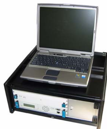
(f) Rack operating on its side with laptop to run CMS software
