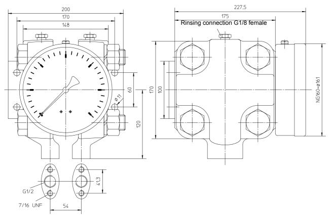
Differential Pressure Gauge DA01 Model: Range (60 ... 400) mbar
