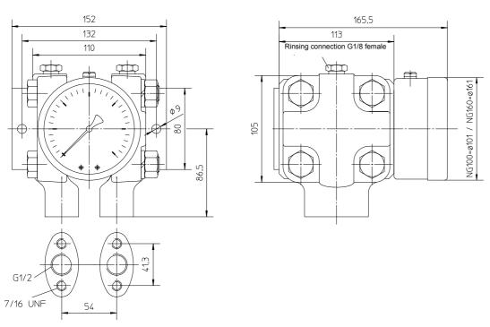
Differential Pressure Gauge DA01 Model: Range (0.6 ... 25) bar
