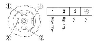
M12 Circular plug connector DIN EN 61076-2-101
