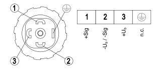
M12 Circular plug connector DIN EN 61076-2-101
