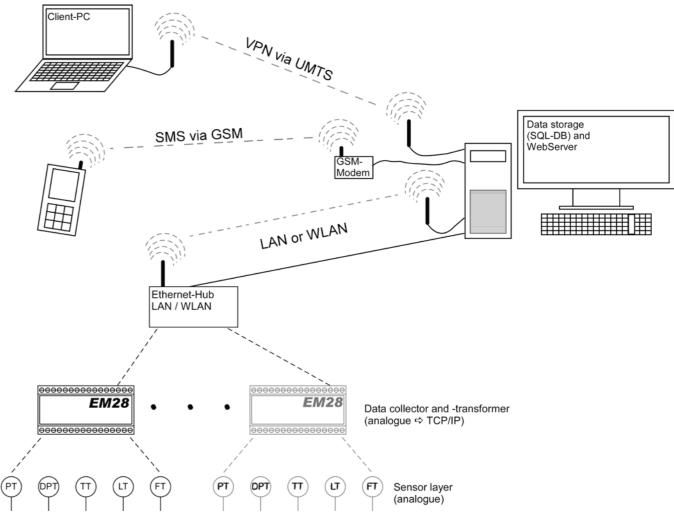
Wireless transmission of measurement signals is available for particularly difficult to reach measurement points.
