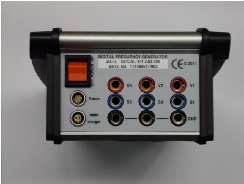
Figure 4 IST-101-A03 Three channel speed calibrator Top View.
