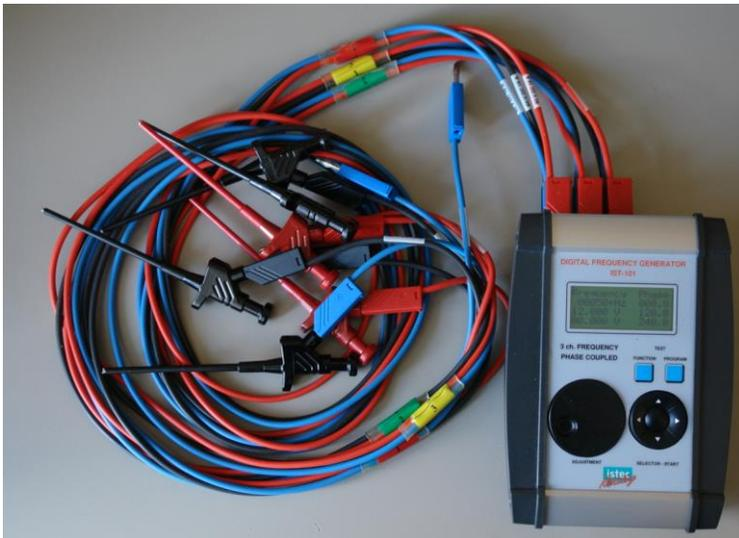
Figure 1 IST-101-A03-XXX Three channel speed calibrator with connection cables.
