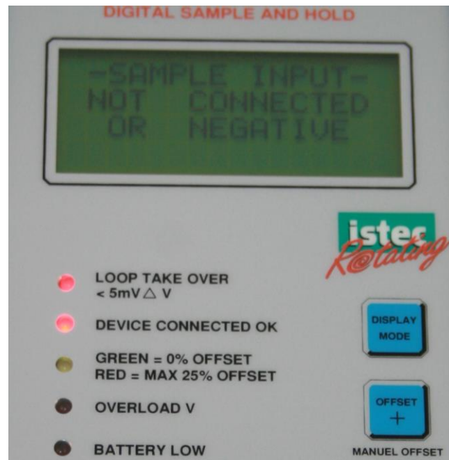
Figure 9 IST-201-A01 / IST-202-A01 Hot Cut Over Tool Display and Status LED's.
