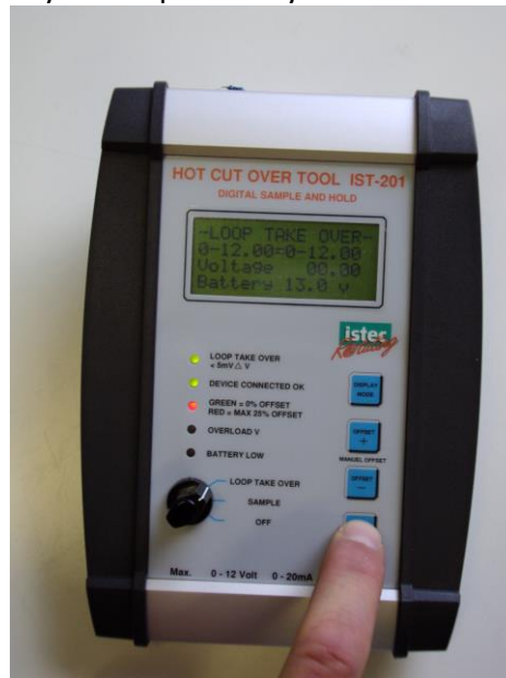
Figure 7 IST-201-A01 / IST-202-A01 Hot Cut Over Tool Battery load.
