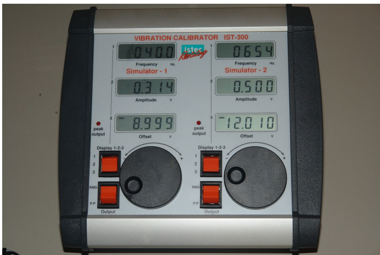
Figure 3 IST-300-A02 Two channel calibrator Front View.
