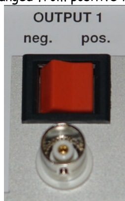
Figure 10 IST-300-A02 Two channel calibrator Polarity Switch
