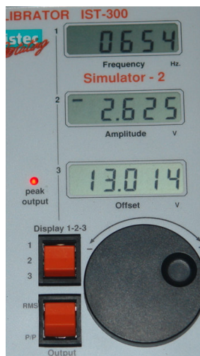
Figure 12 IST-300-A02 Two channel calibrator Peak Output Function
