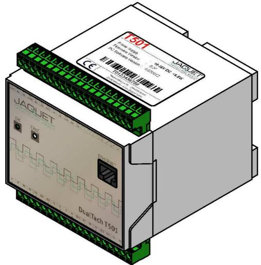
**T501 :** 2 Channel Tachometer with 4 Relays and 2 Analog Outputs 0/4-20mA **T501.50:** Part No.: 384Z-05600 (AC Version) **T501.10:** Part No.: 384Z-05601 (DC Version)
