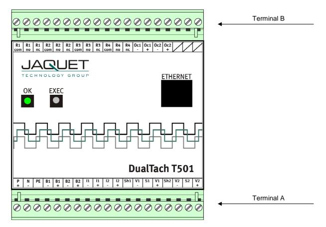
The Ethernet Interface, status LED along with the EXEC push buttong are located at the front. For communications please see Paragraph 7 Configuration via PC Software
