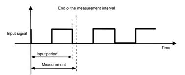
If the input period is greater than the measurement interval, the frequency is calculated as follows:
