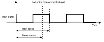
The calculation and adjustment of outputs occurs immediately after the start of the next measurement interval. If the input frequency is lower than the lower limit (0.025Hz), then the output will be zero. The measurement of input frequencies above the upper limit (50kHz) is not guaranteed.
