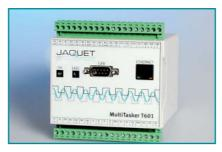
MultiTasker with 2 frequency, 1 analogue & 2 binary inputs; 2 analogue, 4 relay and 2 open collector outputs; CAN bus and Ethernet interfaces; Event recorder and trip data-logger; for complex measurement, control, protection and communication.
