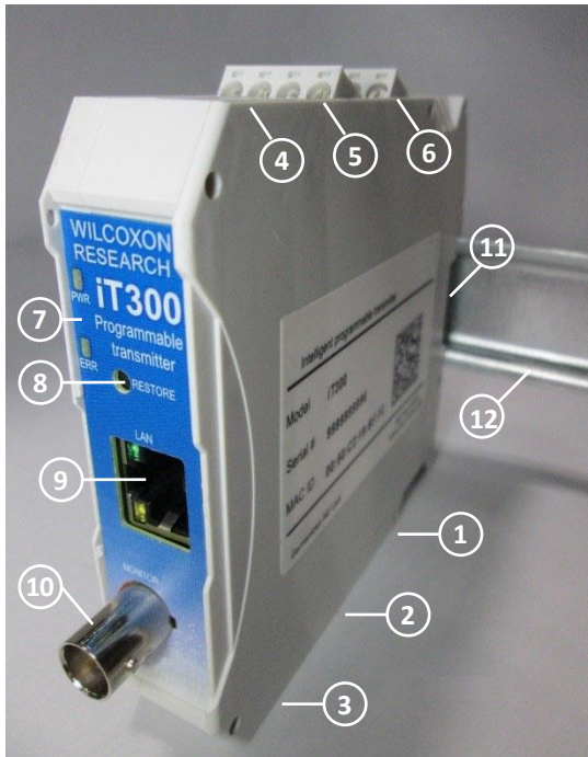
Figure 1 - Major system components
