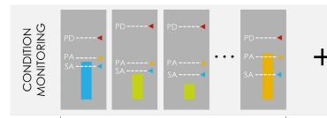
Protection measurements and statuses **shared** with CM system (**not re-created**) and **augmented** with additional SW-only alarms (SA)
