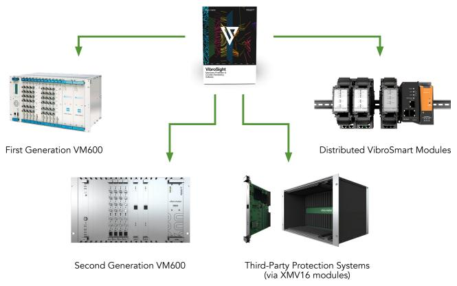
VibroSight integrates various hardware platforms – including third-party platforms – into a unified environment for monitoring and managing machinery condition.
