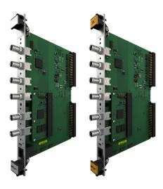
The first-generation VM600 platform was available with both standard and SIL 2 versions of protective modules as shown above. VM600<sup>Mk2</sup> will likewise be available with SIL 2 versions of protective modules (MPC4<sup>Mk2</sup> and RLC16<sup>Mk2</sup>) later in 2022.
