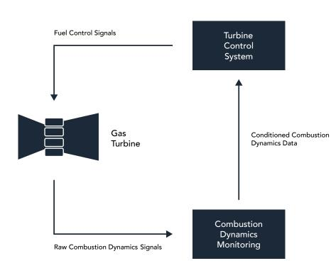
Combustion dynamics monitoring is part of closed-loop control to ensure that damaging pulsations in low-NOx gas turbines do not prematurely age or destroy the combustor cans. The pulsations occur because today's low-NOx technologies rely on inherently metastable combustion conditions that burn fuel in the leanest possible manner but can produce an unstable flame if not meticulously controlled.
