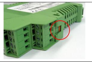
To open press both locking tabs with a screwdriver and then pull out the upper side of the housing.
