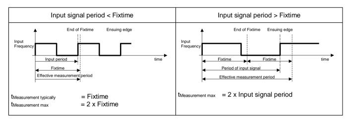
The total measurement time has a resolution of  $\pm$  0.4  $\mu$ s.
