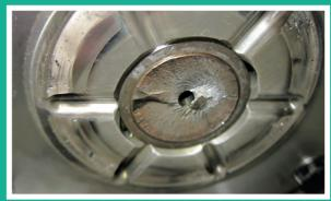
Fatigue crack - pump side
