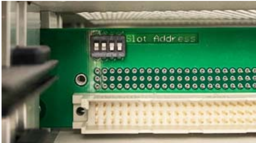
(a) Location of DIP switch on the rack's backplane – rear of rack, top left (accessible when the cards are removed)
