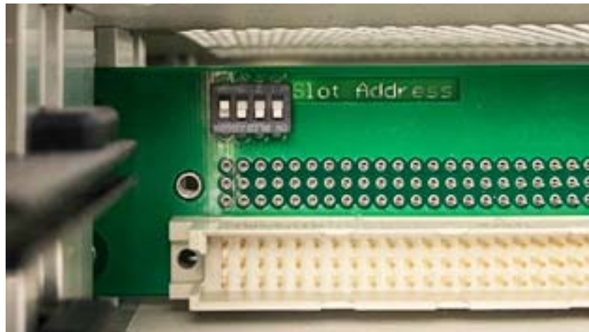
(a) Location of DIP switch on the rack's backplane – rear of rack, top left (accessible when the modules are removed)
